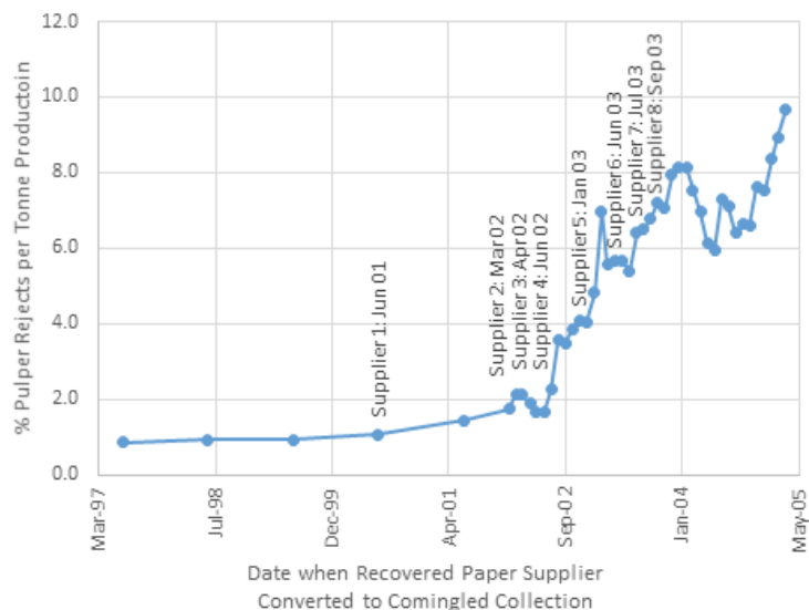
Figure 9: Mill losses increase as suppliers convert to comingled collection (Sacia and Simmons 2006)
